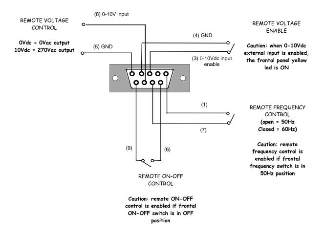
WARNING!: During REMOTE CONTROL situation, please turn the frontal knob in the minimum output voltage level.
