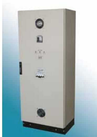
The "RTG" series automatic voltage stabilisers feature independent control of each phase to permit constant voltage regulation even in presence of highly unbalanced loads. Three electronic control circuits, six servomotors and six variable transformers guarantee high level performance and reliability.
