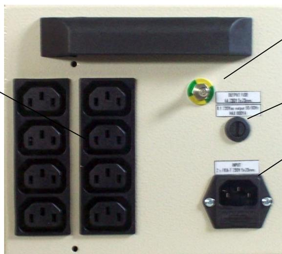
Output sockets, to be used with the special cables with IEC60320 plug. The total load must never exceed the maximum power of the unit
