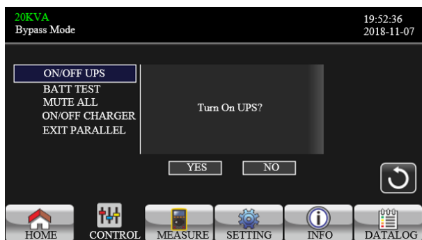
TURN ON UPS
